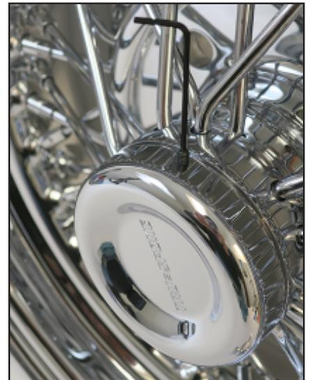
**Above and below:** Twist-on your Spinner or Donut cap until it is tight. Once the cap is tight, tighten each set screw until the screws are tight. Do not over-tighten the screws or they may strip. Make sure you cannot move the cap by hand. Once you have verified your cap is tight, you are finished. Enjoy!
