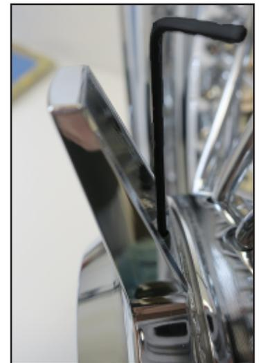
**Special note on the 3-Blade Spinner:** Do not tighten your set screws all the way until after your lug nuts have been installed. You must be able to rotate the spinner to be able to tighten your lug nuts. Once your lug nuts have been tightened, you may finish tightening down your three set screws. Make sure your spinner cap is tight and cannot be moved. Please email or call us with any questions or comments. **Thank you.**
