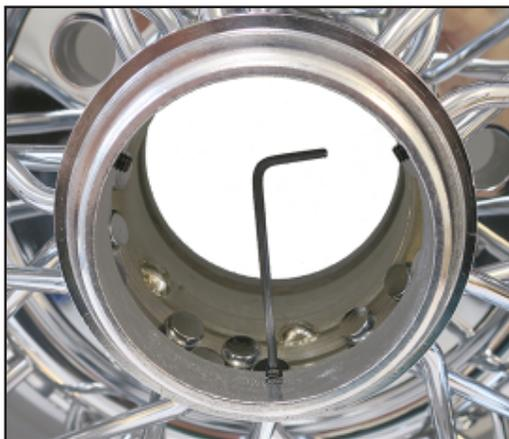
**Above:** Once the tower is in place, using the provided Allen wrench, tighten each set screw equally until they are tight and the tower cannot be moved. **Make certain that the tower is inserted as far as it will go before tightening the screws.**
