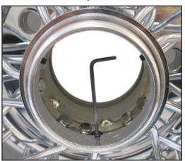
The 3-Bar Spinner has three set screws, one under each blade. Tighten the set screw part way before installing it onto the tower.
