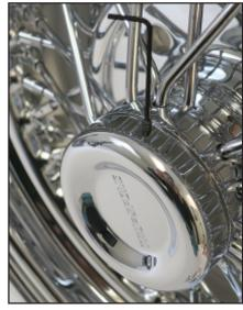
Above and below: Twist-on your Spinner or Donut cap until it is tight. Once the cap is tight, tighten each set screw until the screws are tight. Do not over-tighten the screws or they may strip. Make sure you cannot move the cap by hand. Once you have verified your cap is tight, you are finished. Enjoy!
