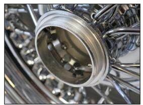
AFTER your wheel and tire have been mounted and balanced, place the tower into the center of the wheel hub as shown. Make sure the tower is fully inserted and seated.
